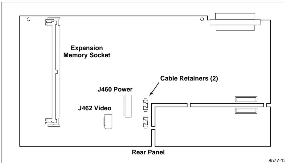
**Figure 7. Connector and Cable Retainer Locations**
