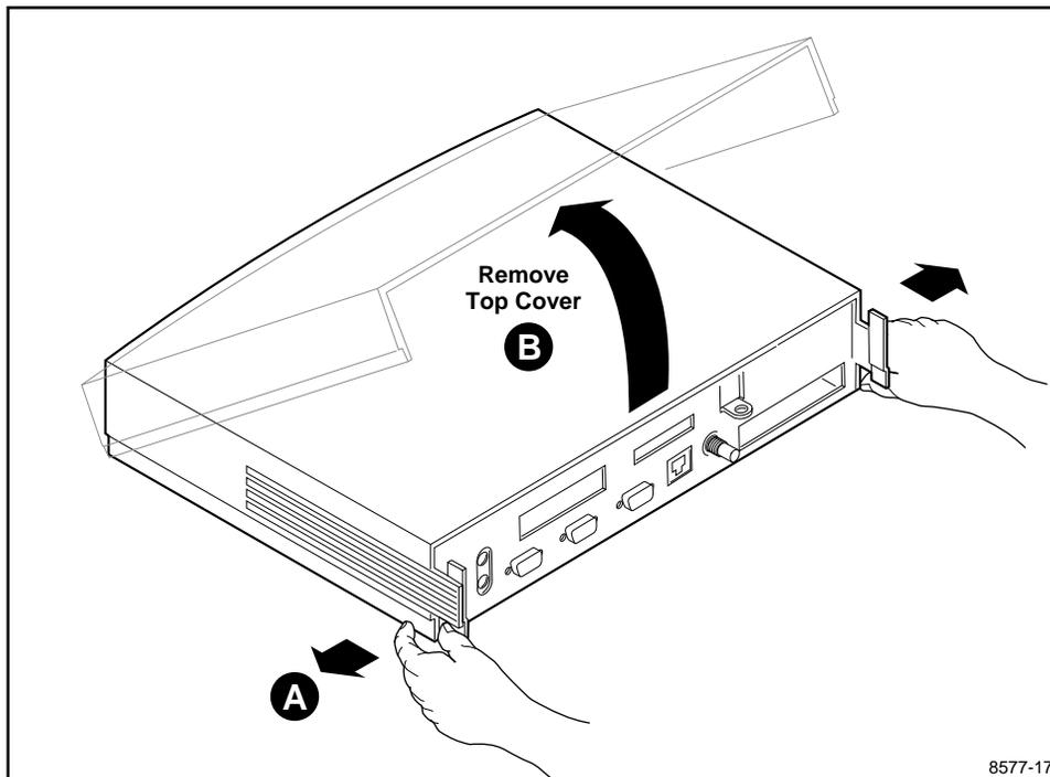
Figure 22. Removing the Pizza Box “C” Logic Module Cover
