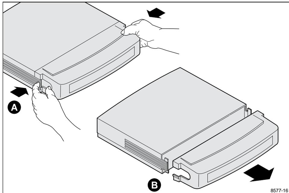
**Figure 21. Removing the Cable Cover**
