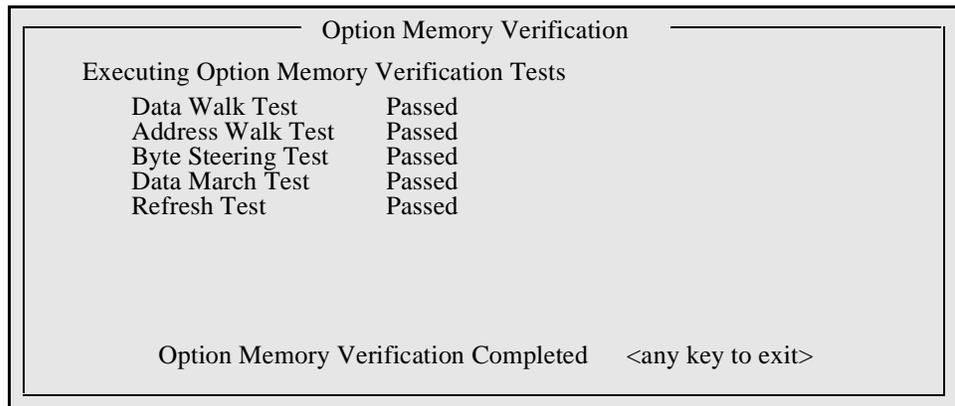
**Figure 27. Screen Display After Successful Expansion Memory Verification Test**
