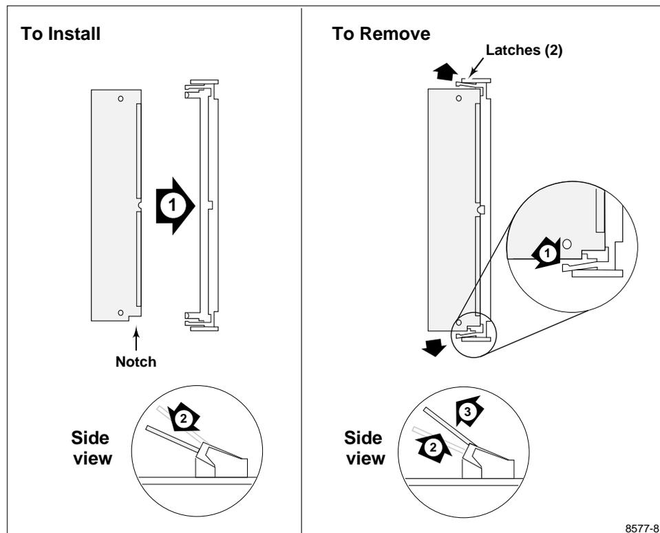
**Figure 8. Installing or Removing the Memory Board**
